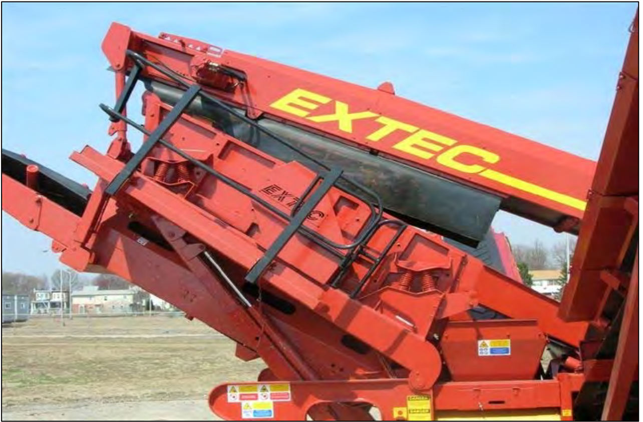
Screen box in working position max angle 34°
