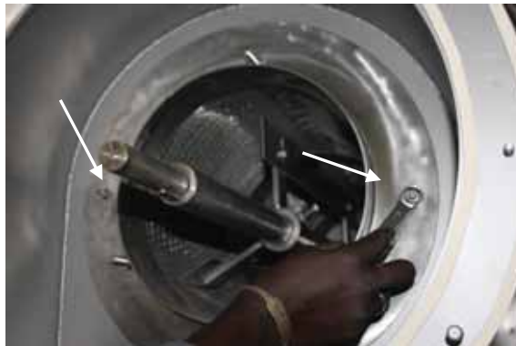
Fig. 6.2 two bolts holding into position the cylindrical net
