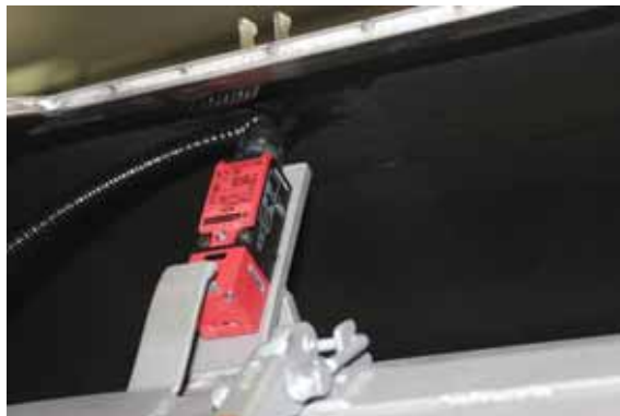
Fig. 2.1 Safety device "closed" - rotative separator working
