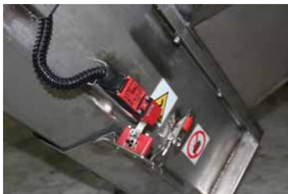
Fig. 2.3 Safety device on the auger screw cleaning door
