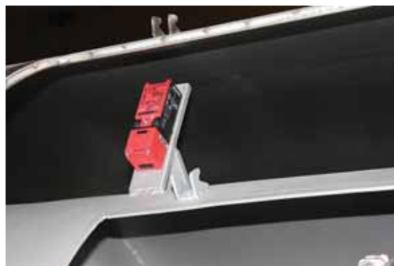
Fig. 2.2 Safety device "opened" - rotative separator stopped
