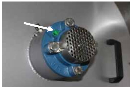
Fig. 6.1 Grease nipple of the grinder/shredder
