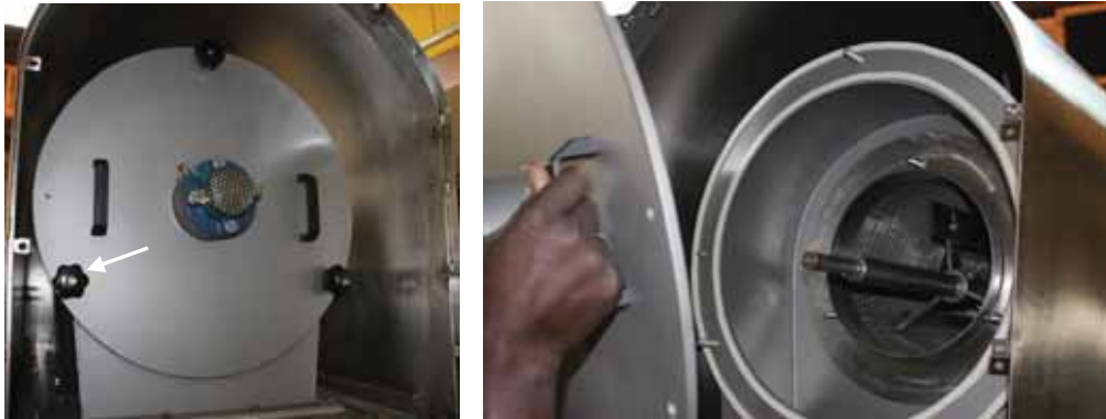
Fig. 6.2 internal bearing support cover removal
