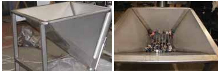
Fig. 3.1 Feeding auger screw hopper with the grid
